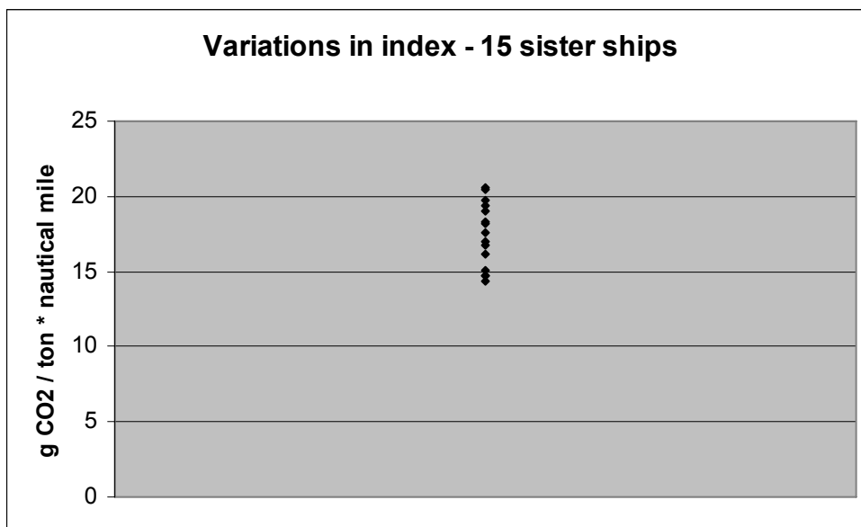
Figure 19 Index value calculated over a period of one year for 15 sister ships
